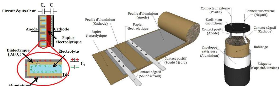
Figure 1 Schematic representation of an electrolytic capacitor.
