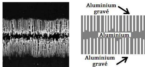
Figure 2: SEM cross section observation of a tunnel pits structure of the anode.
